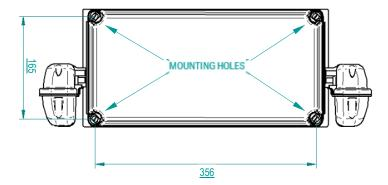
Note: This diagram shows the LWP2LIFE-PRO-WPPOD in the wall mount configuration with the PODs rotated down. To mount to the ceiling using the same mounting instructions but ensure the heads are facing down
